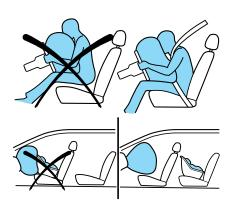
**WARNING:** All occupants of the vehicle, including the driver, should always properly wear their safety belts, even when an air bag supplemental restraint system (SRS) is provided.
